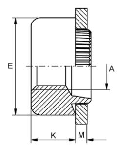
Female thread A = M3,5 Height K = 4.0Outer diameter E = 10.0Plate thickness = 1.4 to 1.6
